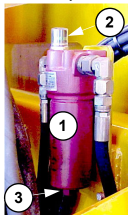
Photo 15 Hydraulic oil filter lateral movement circuit
